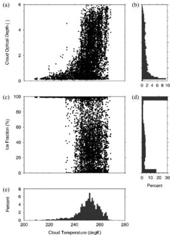
Figure 4. Optical depth and ice fraction of single layer clouds November 1997 to May 1998 at SHEBA. Optical depth scatter plot versus cloud temperature (a), and occurrence histogram (b). Ice fraction versus cloud temperature (c), and occurrence histogram (d). Frequency distribution of cloud temperatures (e) (from Turner, 2005).
