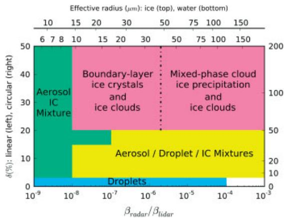
Figure 3. Classification of wintertime atmospheric particles and their mixtures from Eureka, 2005–2008. Effective radii for liquid droplets and spherical ice crystals (IC) are calculated for a given colour ratio, although this is only valid where there are no aerosols (from Bourdages *et al.*, 2009).
