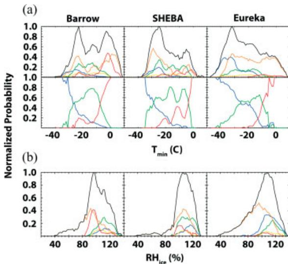
Figure 10. Normalized occurrence probability distributions of different cloud types as a function of temperature (a) and relative humidity (b) over ice for three Arctic sites. Distributions are for total cases (—), clear sky (—), ice clouds (—), liquid clouds (—), mixed-phase clouds topped by water (—), and ice-topped clouds with mixed-phase layers (—) (from de Boer *et al.*, 2011).
