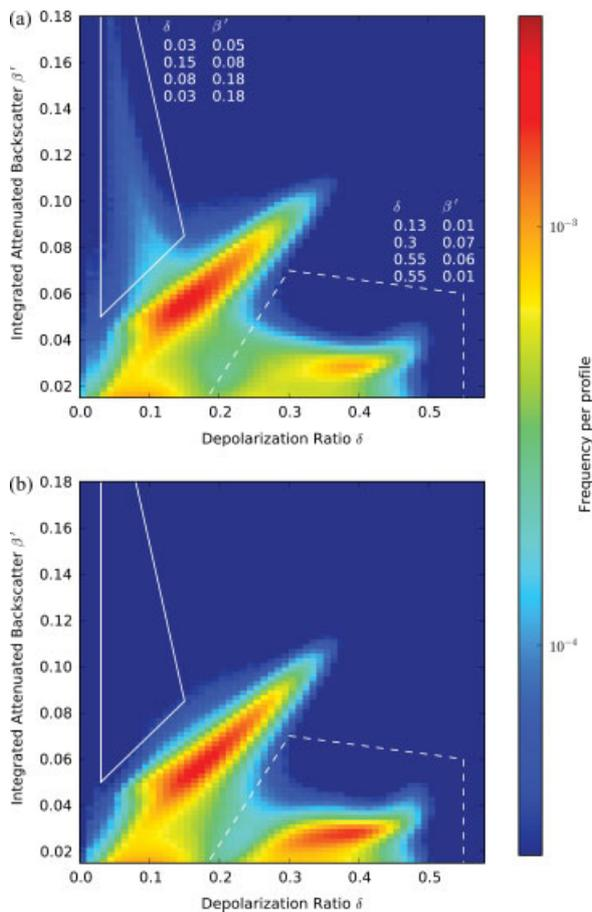
Figure 6. Integrated backscatter/depolarization ratio distributions of on-nadir (a), and off-nadir (b), global cloud returns from CALIPSO. The area outlined by the solid line indicates aligned ice while that outlined by the dashed line indicates randomly oriented ice. Coordinates of these regions are given in (a) (adapted from Noel and Chepfer, 2010).
