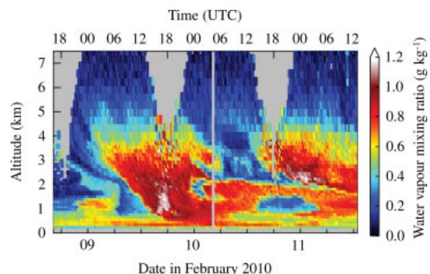
Figure 11. Water vapour mixing ratio measured at Eureka, February 2010. Gray regions indicate invalid or missing data (adapted from Doyle *et al.*, 2011).
