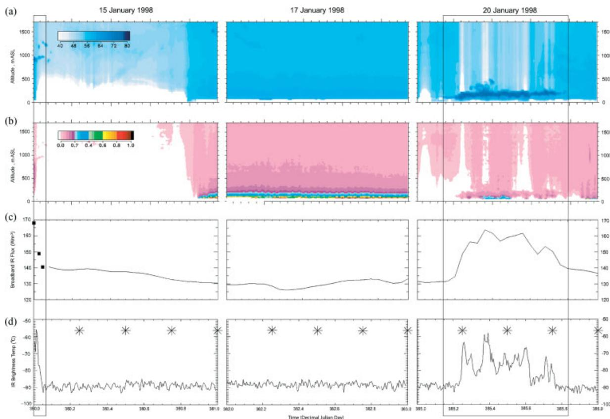
Figure 8. Lidar backscatter (a), and depolarization ratio (b), of instances of diamond dust recorded in January 1998 during SHEBA. Coincident long wave irradiance (c), and brightness temperatures (d), show that only when the ice crystals are associated with cloud (indicated with the black vertical lines) is the radiation affected (from Intrieri and Shupe, 2004).
