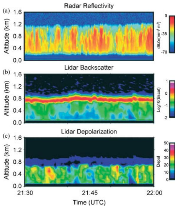
Figure 5. Cloud radar reflectivity (a), lidar backscatter (b), and lidar depolarization ratio (c) of a single layer mixed-phase cloud measured during M-PACE. Note that the lidar signal is fully attenuated before reaching the cloud top at 1.2 km (from Verlinde *et al.*, 2007).
