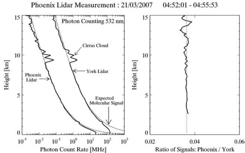
**Figure 4.** Atmospheric measurements obtained simultaneously with the Phoenix lidar and the York Lidar at the wavelength of 532 nm. The Phoenix lidar was operating inside the thermal vacuum chamber in an environment consisting of carbon dioxide at a pressure of 8 torr and a temperature of  $-70^{\circ}\text{C}$ . The Phoenix lidar internal chassis temperature was  $-36^{\circ}\text{C}$ .
