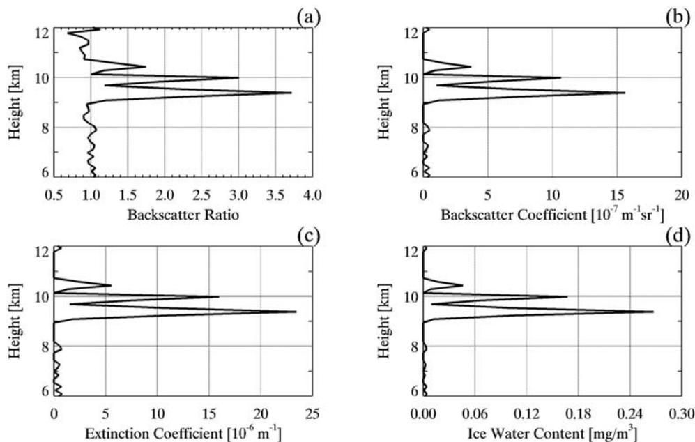
**Figure 6.** Four steps in the analysis of lidar data applied to the cloud backscatter signal in Figure 4.
