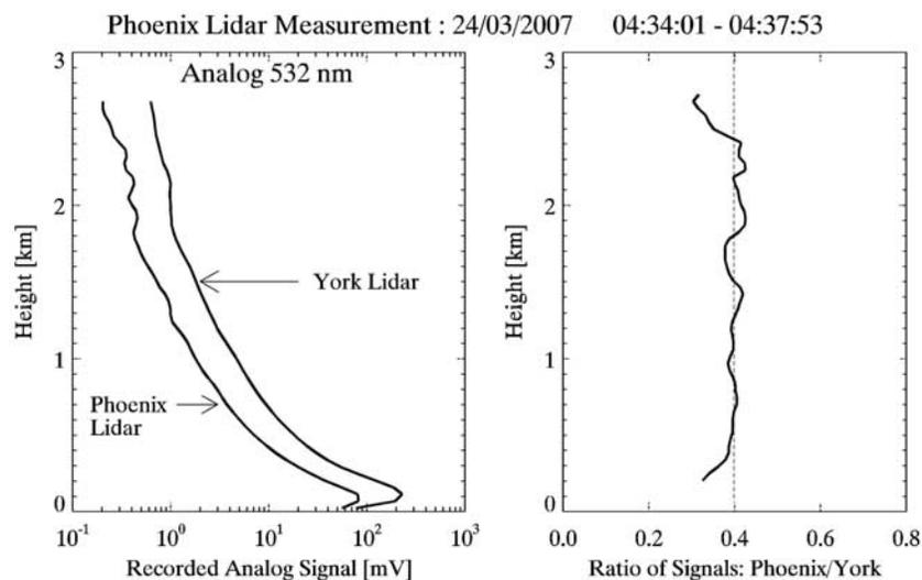
**Figure 5.** Atmospheric measurements obtained simultaneously with the Phoenix lidar and the York Lidar at the wavelength of 532 nm and recorded by analog to digital conversion. The Phoenix lidar was operating inside the thermal vacuum chamber in an environment consisting of carbon dioxide at a pressure of 8 torr and a temperature of  $-70^{\circ}\text{C}$ . The Phoenix lidar internal chassis temperature was  $-30^{\circ}\text{C}$ .
