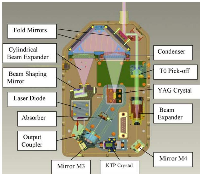
**Figure 3.** Drawing of the Phoenix lidar laser transmitter.
