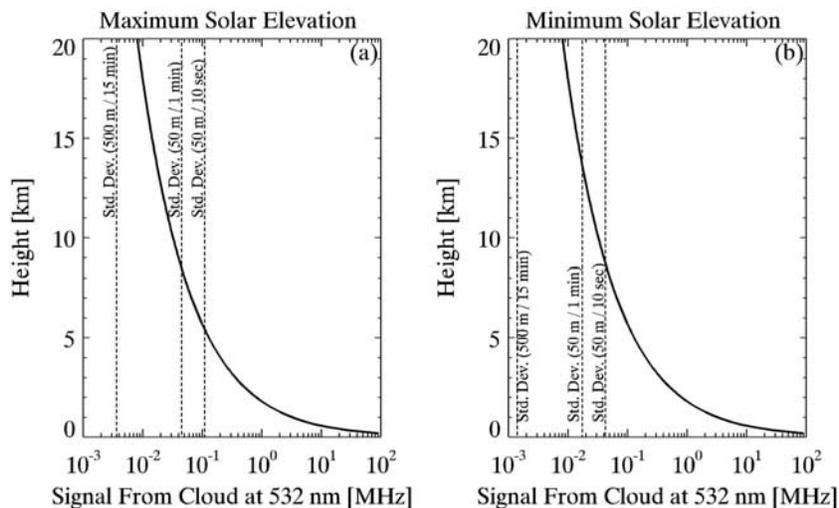
**Figure 7.** The 532 nm photon counting backscatter signal from a cloud equivalent to the one in Figure 4 (solid) compared with the standard deviation of the statistical fluctuation in the background skylight signal (dashed).
