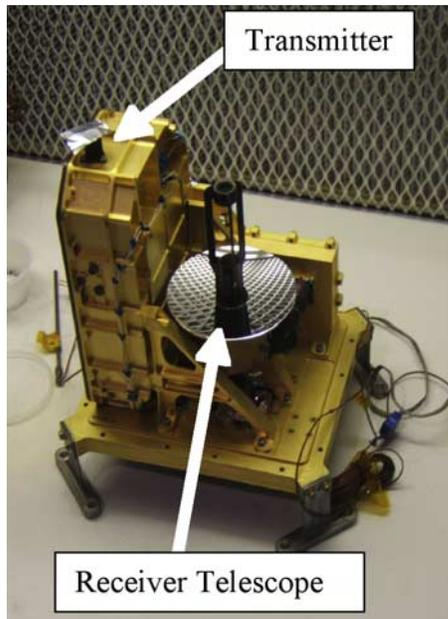
**Figure 2.** Photograph of the Phoenix lidar with the cover removed.
