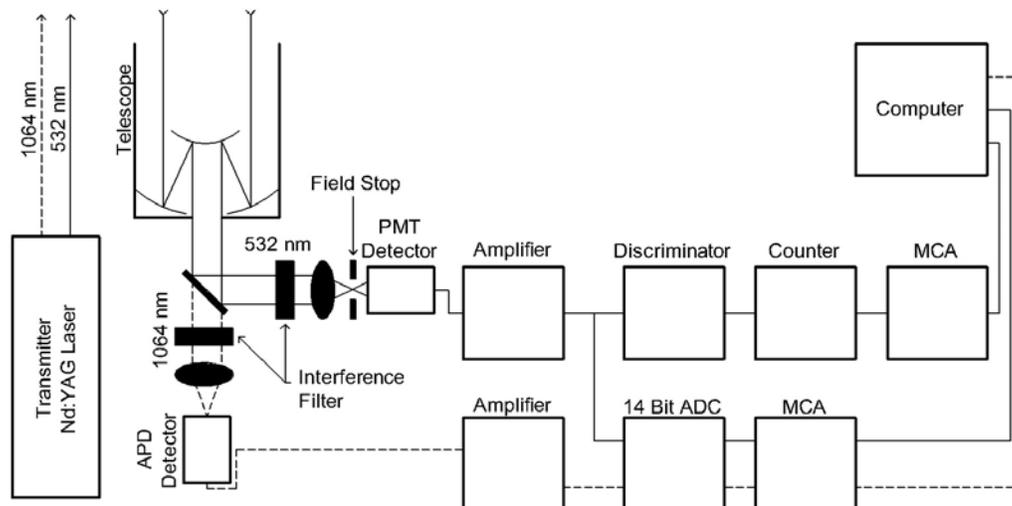
**Figure 1.** Schematic diagram of the Phoenix lidar.
