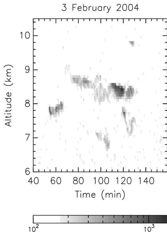
Fig. 2. A measurement of range-squared corrected backscatter obtained on 3 February 2004. The measurement shows the extent and structure of a high-altitude cloud.
