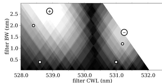
Figure 3: Temperature sensitivity versus filter bandwidth and center wavelength in arbitrary units (white is  $\pm 1$ , black is 0). Squares are for daytime filters, circles are for the night time filter set.
