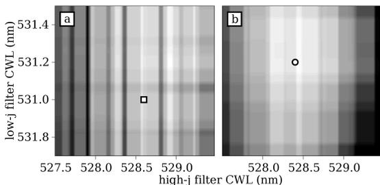
Figure 4: Temperature uncertainty versus filter center wavelength in arbitrary units (white is 0, black is 1) for daytime, (a), and night time, (b), filters.
