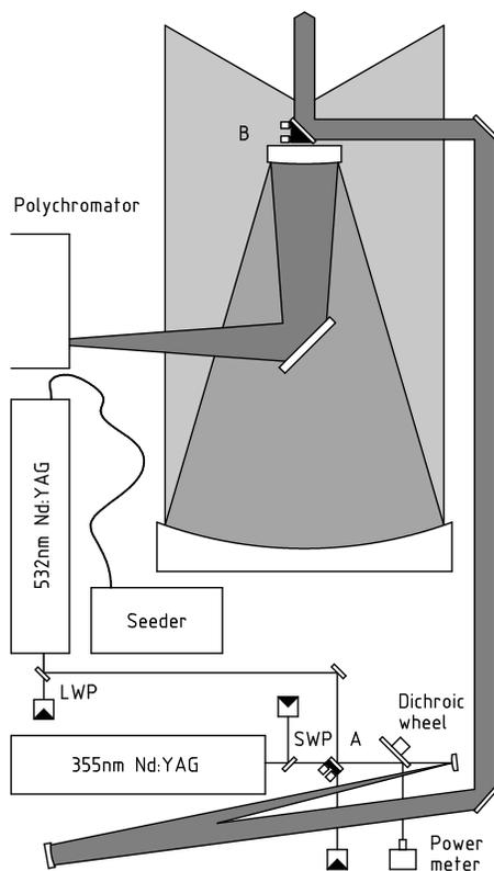
Figure 1: Schematic of the lidar. A long-wave pass dichroic (LWP) removes the residual NIR while a short-wave pass (SWP) removes residual visible and NIR from the UV beam. Dichroic A is a SWP that coaligns the green and UV beams and has stepper motor actuators to align the green beam to the telescope FOV. After expansion, a final 4" mirror, B, is used to steer the UV beam into the telescope FOV. See section 2.1 for details.
