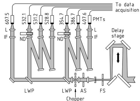
Figure 2: Schematic of the polychromator receiver chain. FS is the field stop, AS the aperture stop. Long wave pass dichroics, LWP, split the light into UV and visible arms and separate the  $N_2$  Raman line from the shorter visible channels. ND are neutral density filter wheels. Each channel has an interference filter, IF, and lens, L, to focus light onto the PMT.
