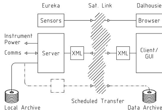
Figure 5: Simplified lidar control software structure. See text for details.
