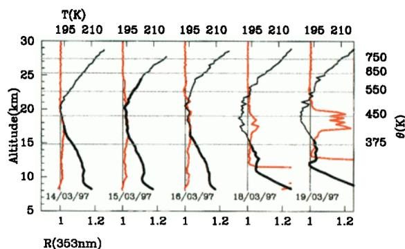
**Figure 4.** Scattering ratio ( $R$ ) profiles in red along with the lidar derived temperature profile (blue) and sonde temperature profile (black). The vertical line denotes  $R=1$  and  $T=193 \text{ K}$ . The large increases in  $R$  near the tropopause for the 18-19th are caused by the presence of cirrus clouds.
