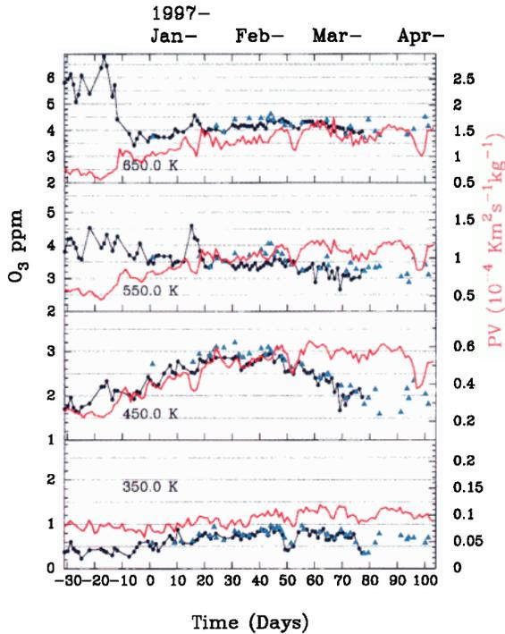
**Figure 1.** Lidar derived ozone mixing ratio (dark blue), ozone sonde measurements (light blue triangles) and CMC potential vorticity (red) for different potential temperature levels. The values shown are averages over  $\pm 50$  K about the  $\theta$  levels shown.
