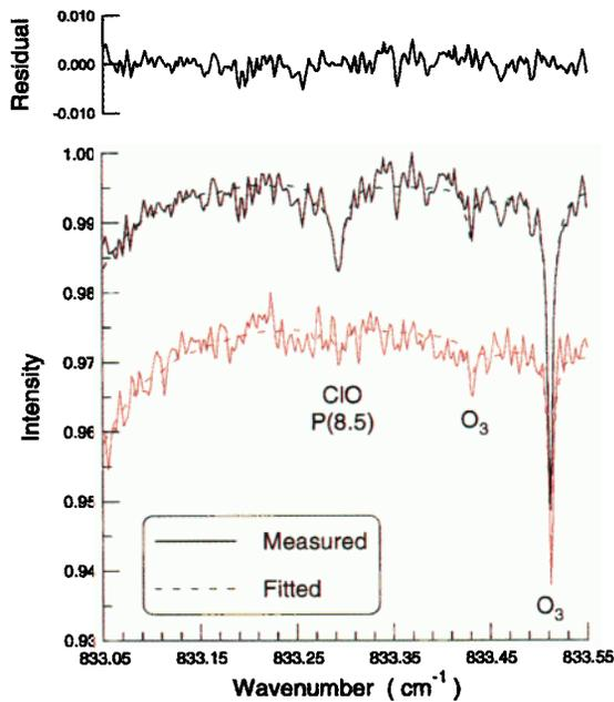
**Figure 5.** The spectral fit obtained in the region of the P(8.5) ClO line recorded on 27 February, 1997, at a solar zenith angle of 88.8 degrees. The residuals for this fit are plotted immediately above. In red and shifted down, the spectrum recorded on 20 March, 1997 is shown for comparison.
